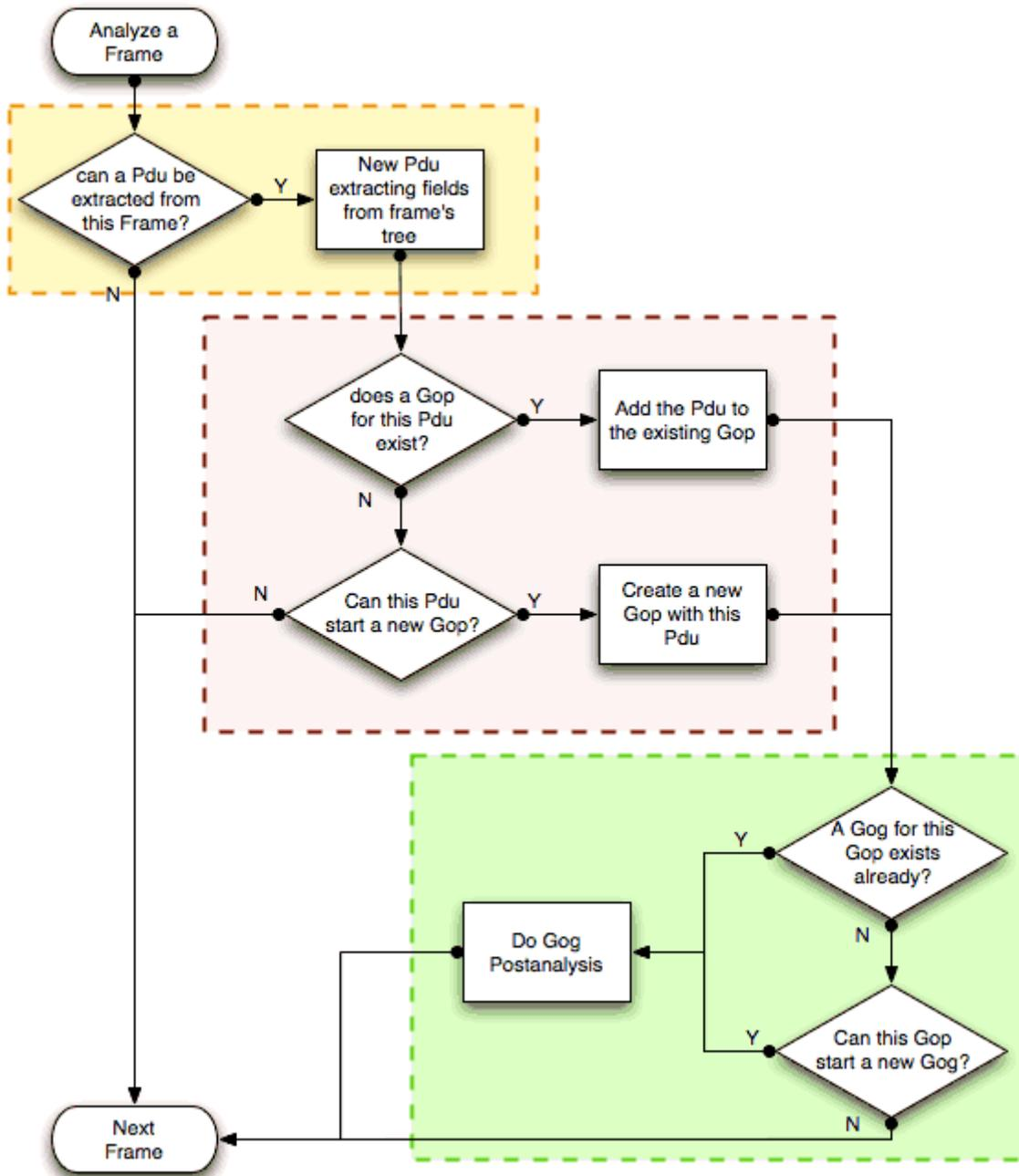
Figure 140. MATE Analysis (PDU → GOP → GOG) flowchart
