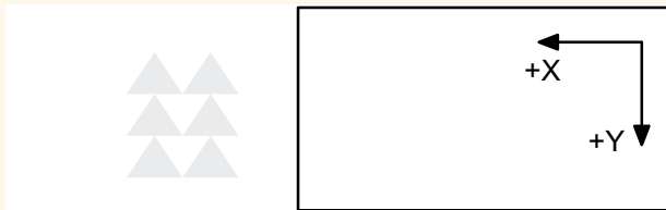
Figure 165. HP-GL/2 Pattern Orientation for Plotters with Landscape Layout
